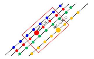
**Figure 3.** Sketch map of the planes fitted to ground tracks of GLAS. Different colors of footprints denote different tracks. The points A and B are enlarged footprints characterized by their coordinates (E, N, H) and acquisition time (t). The red window shows the sampled facet.
