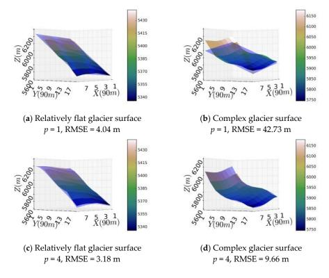
**Figure 5.** (**a**,**b**): the fitted surface and real surface when p = 1; (**c**,**d**): the fitted surface and real surface when p = 4. The light blue surface represents the fitted surface and the gradient colored surface represents the real surface.
