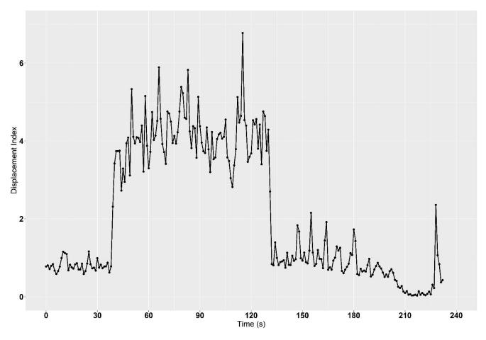
**Figure 5.** This small extract of a delivery (t = 232 s) shows an access road to a sow farm. On this road section, vibration emissions with a Displacement Index ( $D_i$ ) > 3 are recorded during a time span of 90 s. Dots on the chart line represent single measurement points of  $D_i$ -values.
