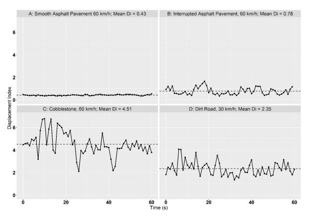
**Figure 2.** Exemplary Displacement Index curves for selected test runs. Dots on the chart line represent single measurement points of  $D_i$ -values, and the dashed line shows the mean Displacement Index  $(D_{\overline{x}})$  of this test run.
