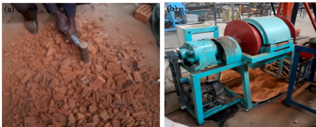
Fig. 1. The process of ball milling: (a) crushing fragmented clay bricks and (b) grinding crushed clay bricks using ball mill.
