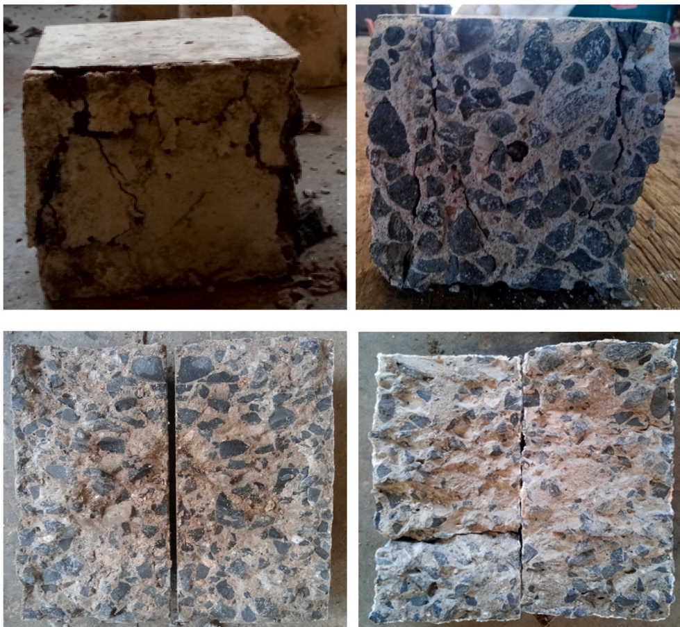
Fig. 20. Cubes and broken cylinder specimens for class 30 (5P0T) concrete mixes after testing: cured using water (left column) and exposed to sulfuric acid (right column).
