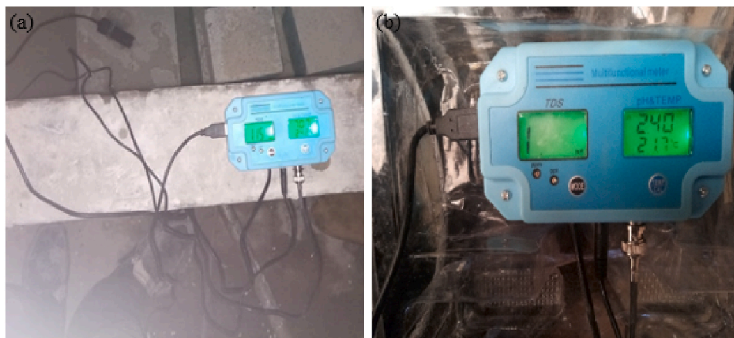
Fig. 8. Monitoring temperature and pH of exposure conditions using a portable pH meter for (a) samples cured in water and (b) samples exposed to sulfuric acid.
