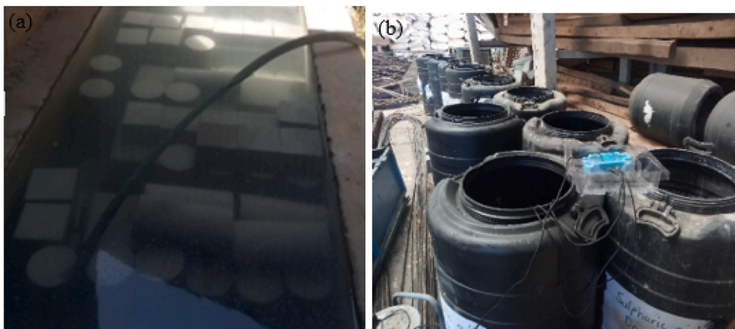
Fig. 7. (a) Concrete curing in water and (b) concrete exposure to sulfuric acid.
