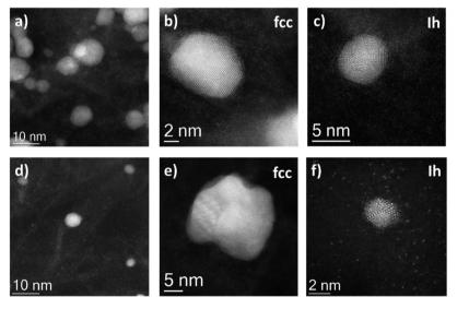
Figure 10.  $C_s$ -corrected STEM-HAADF images of 2-rGO after one catalytic cycle (a-c) and 10 catalytic cycles (d-f). Zooming of the Pd(0) NPs show the fcc crystal nature of some of the NPs (b,e) and the icosahedral (Ih) structures (c,f).
