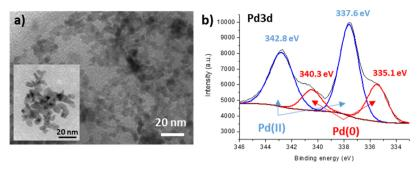
Figure 4. HRTEM image of 2-NPs (a) and XPS analysis (b) showing the presence of Pd(0) and Pd(2+).
