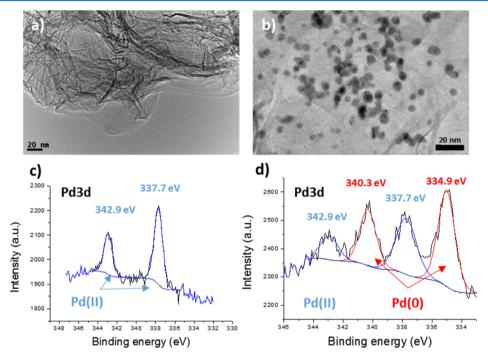
Figure 5. HRTEM images (top) and XPS analysis (bottom) for the core-level peaks of Pd 3d. HRTEM of 2-rGO (a) before and (b) after the exposure to  $H_2$ . XPS analysis of 2-rGO (c) before and (d) after the exposure to  $H_2$  showing the characteristic peaks of Pd(0) and Pd(2+).
