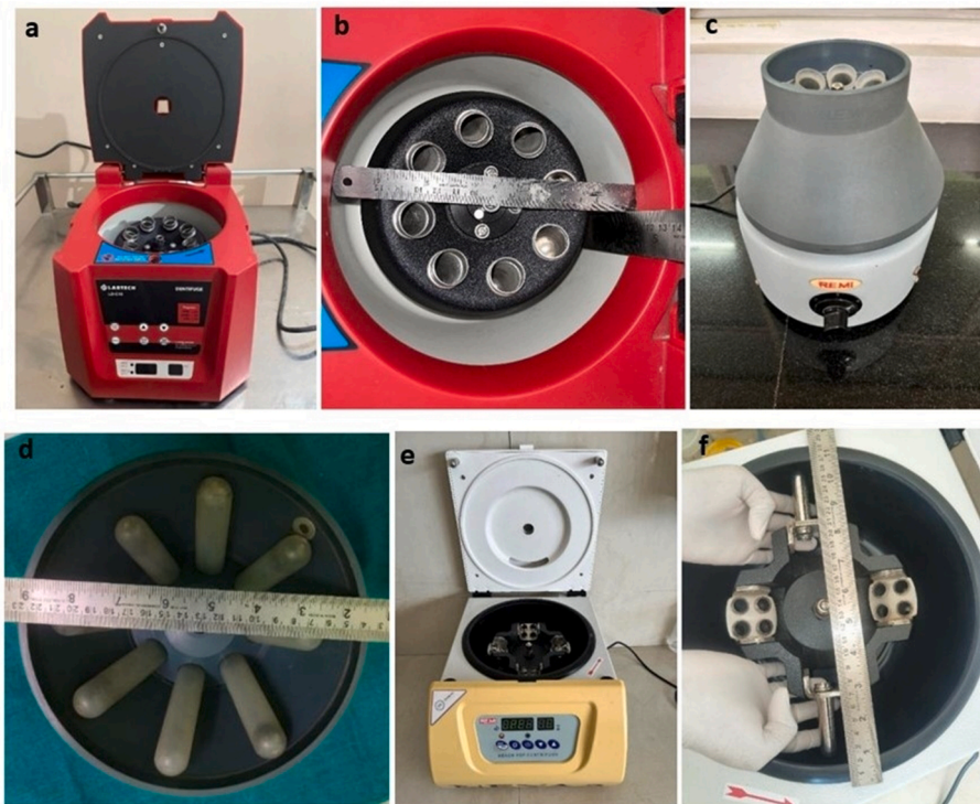
Fig. 1 (a). Labtech Centrifuge with; (b) Fixed rotor of radius of 8 cm; (c): Remi R-303 with; (d) Fixed rotor of radius of 7.5 cm; and (e): Neva-2 (Remi, India) with; (f): Swinging bucket rotor of radius 12 cm.
