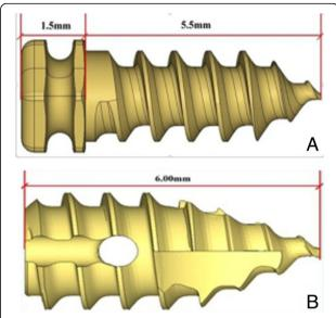
**Fig. 1** The two types of anchoring nails. **a** Traditional anchoring nail. **b** Improved anchoring nail
