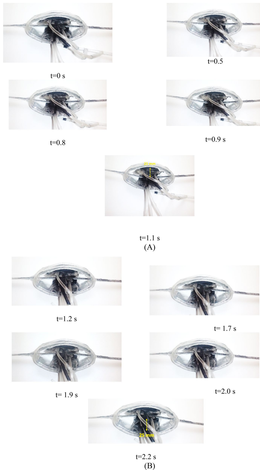
Figure 13. Displacement of the diaphragm over time using two sets of soft actuators up (A) and down (B) directions in HEFR mode.
