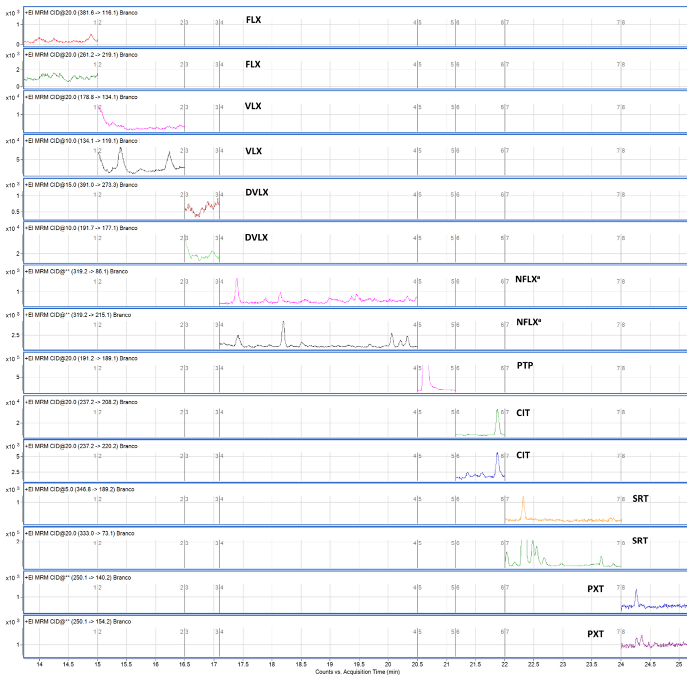
Figure 3. Chromatogram of selected fragments obtained after extraction of a blank oral fluid sample. a : Only for qualitative purposes.
