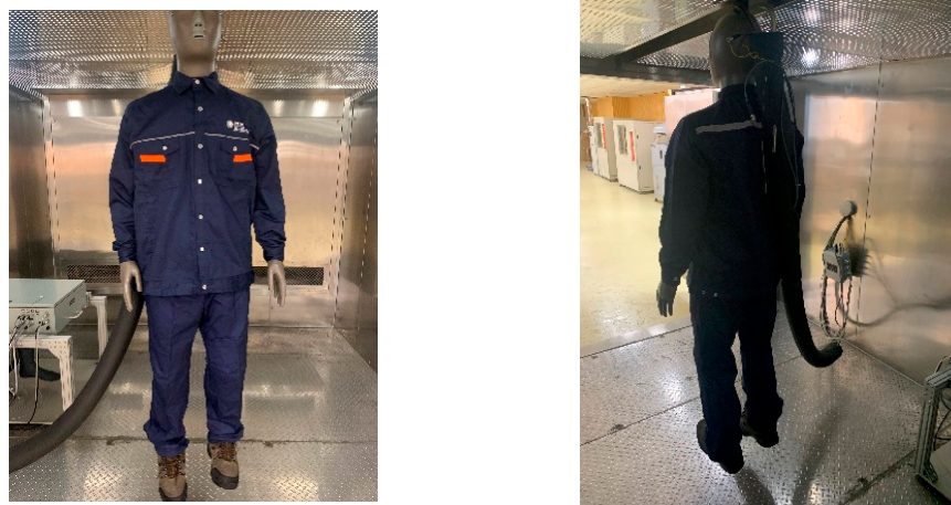
Figure 1. The thermal manikin Newton with power grid ensembles.
