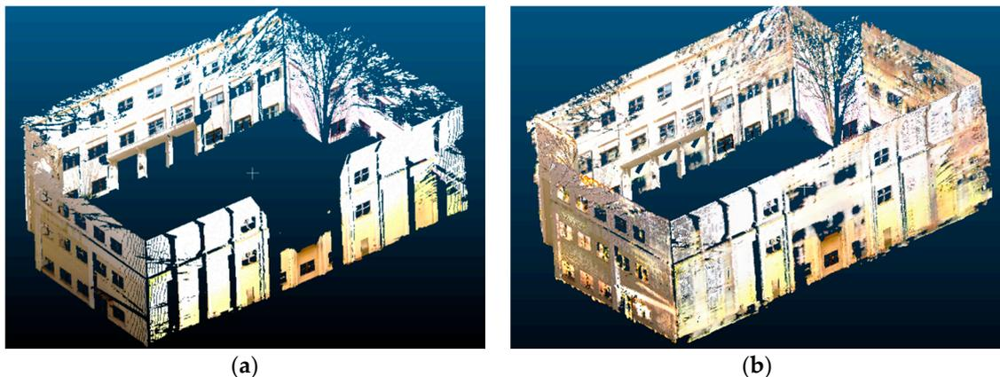
**Figure 13.** Example of 3D scene completion of a full building from partial scans: (a) input point cloud and (b) point cloud result after orthographic projection and generative adversarial inpainting.
