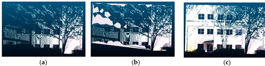
**Figure 16.** Example of a hole-filling limitation. (a) Input, (b) building facade after hole-filling, and (c) target ground truth.
