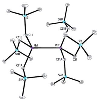
**Scheme 2** The X-ray structure of diplumbane **1** with ORTEP diagram drawn at 30% thermal ellipsoids probability level. Selected bond lengths (Å): Pb1-Pb2 = 2.89922(19), Pb1-C11 = 2.260(8), Pb2-C21 = 2.243(8); and angles (°): C11-Pb1-Pb2 = 115.0(2), C11-Pb1-C11A = 103.5(3), C21-Pb2-Pb1 = 114.2(2), C21-Pb2-C21A = 104.4(3).
