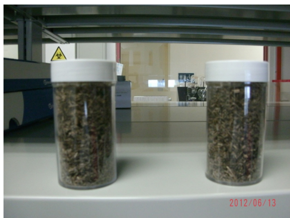
Fig. 1. Washed, dried, and crushed samples of Elaeis guineensis dried midribs.
