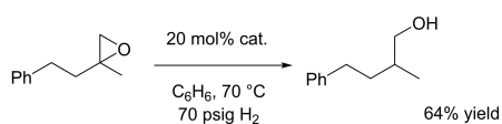
Scheme 14. Catalytic hydrogenation of an epoxide to an anti-Markovnikov alcohol using the \text{Ti}_2\text{Cr}_2 ring compound as catalyst.
