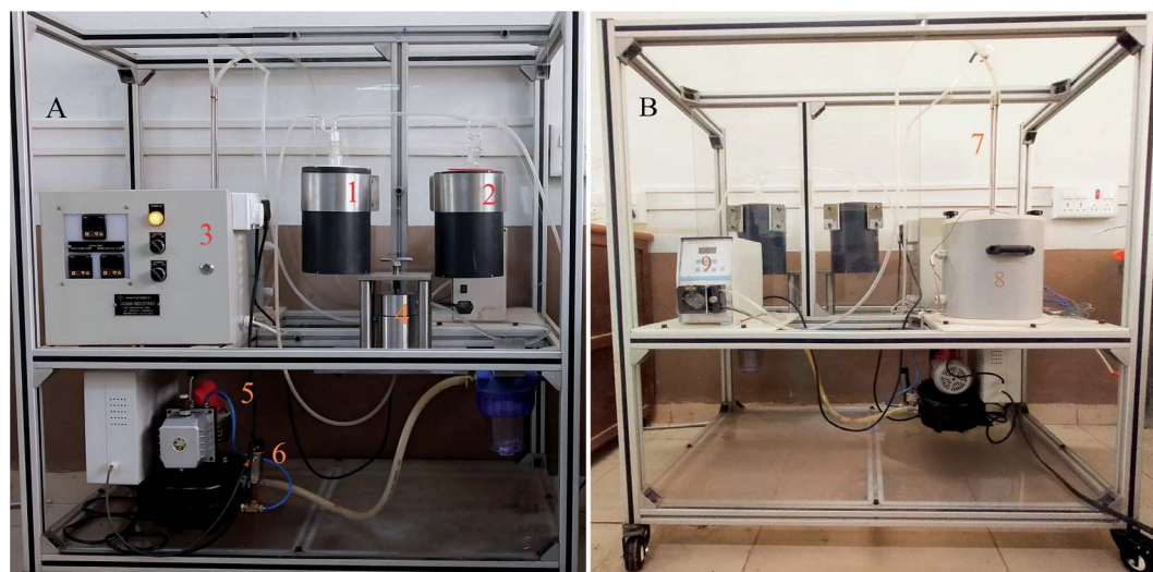
Fig. 2 Photographic image of the pervaporation apparatus: (A) front view: (1) permeate cold trap; (2) moisture cold trap; (3) control panel; (4) pervaporation cell; (5) vacuum pump; (6) vacuum control sensor. (B) Back view: (7) inlet and outlet of the feed tank; (8) feed tank; (9) circulation pump.
