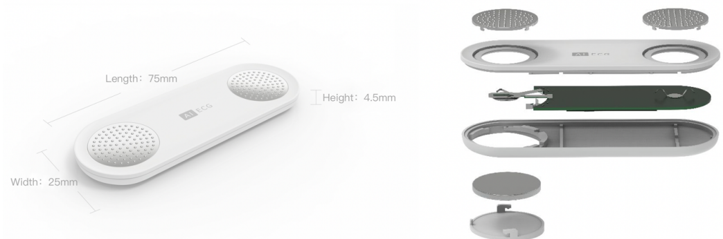
Figure 2. Design of electrocardiogram (ECG) data acquisition hardware.
