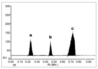
Fig. 1: High performance thin layer chromatograph of standards. High performance thin layer chromatography of Sennoside-A (a), Rubiadin (b) and ellagic acid (c).
