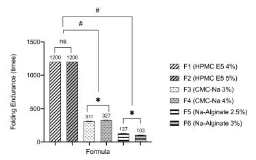
**Figure 2.** Folding endurance in times of the ODFs (mean  $\pm$  SD, n = 4). The (\*) indicates a significant different among similar polymer type groups (p < 0.05); the (#) indicates a significant different between different polymer type groups (p < 0.05); and the (ns) indicates a non-significant different (p > 0.05).
