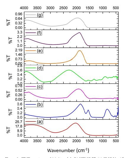
**Figure 9.** FT-IR spectrum of (a) Atenolol; (b) HPMC E5; (c) CMC-Na; (d) Na-alginate; (e) ODF produced from HPMC E5 as film former; (f) ODF produced from CMC-Na as film former; and (g) ODF produced from Na-alginate as film former.
