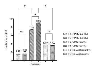
**Figure 3.** Swelling index of ODFs in simulated saliva solution (mean  $\pm$  SD, n = 4). The (\*) indicates a significant different among similar polymer type groups (p < 0.05); the (#) indicates a significant different between different polymer type groups (p < 0.05); and the (ns) indicates a non-significant different (p > 0.05).
