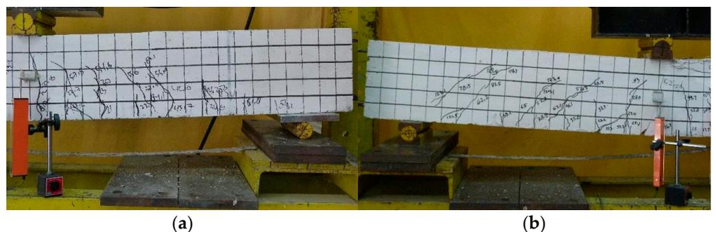
Figure 9. Debonding zone of beams with CFRP plates (a) G6P1, and (b) G6P2.
