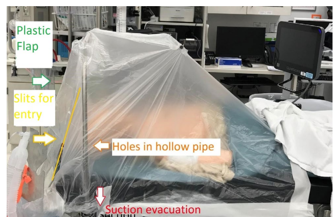
FIGURE 2 Side view of the device with mannequin inside to simulate a patient. Two hollow pipes are used for larger patients with one attached to the right side of the bed to support the plastic in the front and the other attached to the left side of the bed to form the back support [Colour figure can be viewed at wileyonlinelibrary.com ]
