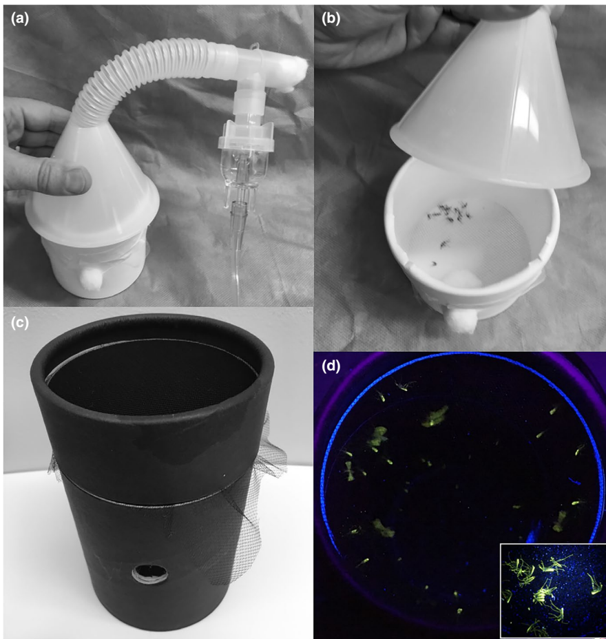
FIGURE 1 Spray Apparatus: Nebulizer and funnel cone over spray cup (a) with mosquitoes (b). Black paper detection cup (c) which limits background fluorescence and allows for detection of live (d) and dead (d inset) fluorescently labelled mosquitoes using a handheld UV flashlight (365 nm). Nebulization technique adapted from Hagler (1997)
