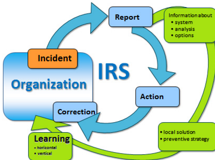
Figure 2: Double function of an incident reporting system. Staff members submit safety-relevant incidents in an anonymised way. The information contained in the report is analyzed and from the multitude of possible reactions a locally feasible solution is chosen. Taken measures or current status of the assessment are communicated to the staff. At the same time care is taken that the knowledge is durably noted in the organization (organizational learning).
