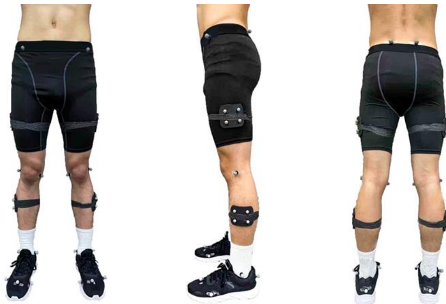
Figure 2. Illustration of retroreflective markers placement.
