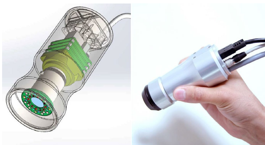
FIGURE 1 Left: Schematic image of the DOE-based spectral imaging device. At the front, the LED illumination ring is shown (color-coded area). The central part holds the DOE-CMOS sensor combination (dark green area), equipped with an appropriate objective. Right: Color image of functional laboratory prototype of the handheld snapshot hyperspectral imaging device [Colour figure can be viewed at wileyonlinelibrary.com ]
