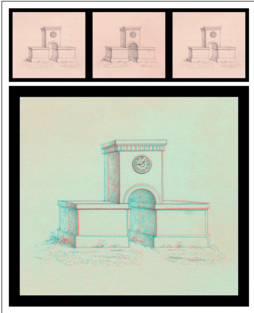
Figure 6. One of the first confirmed stereoscopic images: The Wheatstone Arch (Wheatstone, 1838). Presented in Universal Freeview (L-R-L) format (such that parallel fusion results in a stereoscopic image on the left and a pseudoscopic image on the right, while crossed fusion produces the converse) at the top, and Dubois anaglyph format below.
