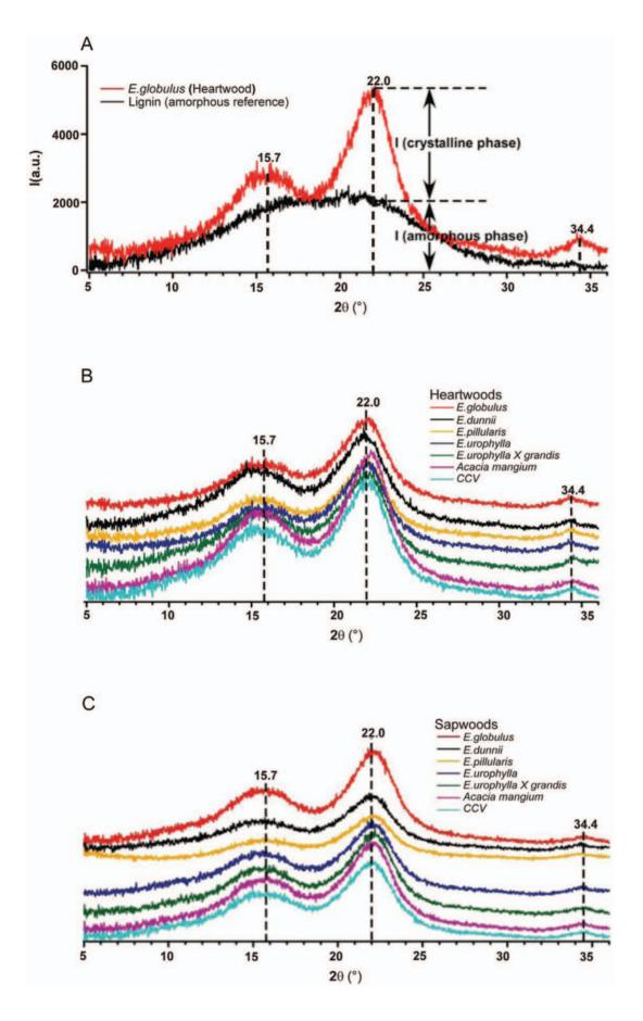
Figure 2. X-ray diffractograms of heartwood and sapwood samples. (A) Example of eucalyptus species (*E. globulus*) and reference (lignin) xray diffractogram to determine amorphous and crystalline phase. X-ray diffractograms of heartwoods (B) and sapwoods (C) of all hardwood species. doi:10.1371/journal.pone.0052820.g002
