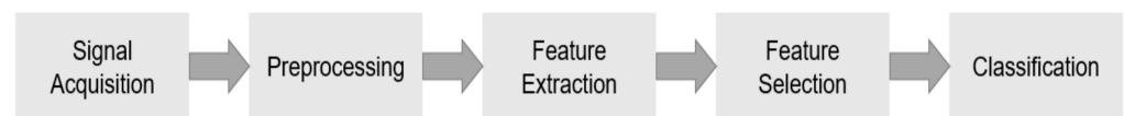
Figure 6. The track an fNIRS-BCI takes in order to receive useable data for an output and the order we will be following to understand the fNIRS-BCI process.
