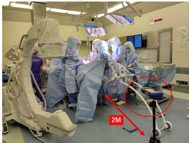
Figure 1. A highly sensitive sound level meter (LA-7500; Onosokki, Kanagawa, Japan) was used to record the hammering sound of stem insertion. In all cases, the sound level meter was set on a tripod mount at 1 meter high and 2 meters away from the surgical table in the same operation room.
