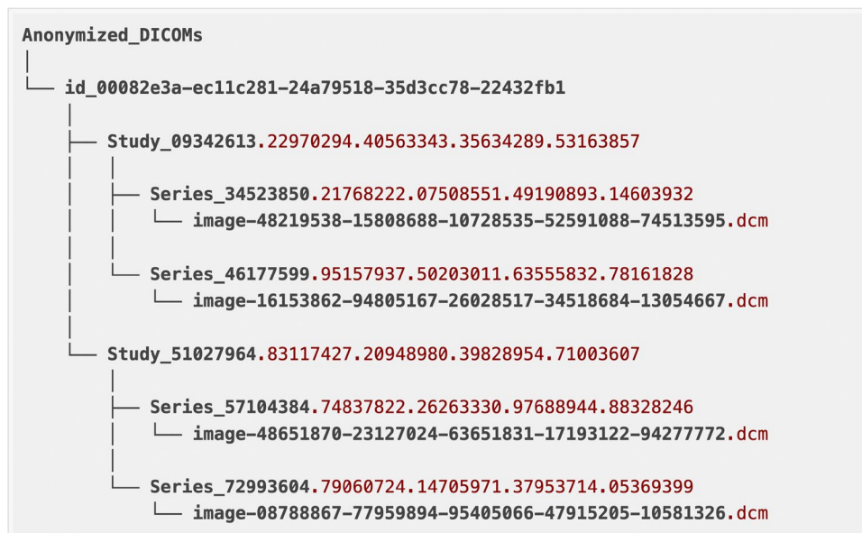
Fig. 6 Example of the Anonymized_DICOMs folder structure for a single patient. Inside the main anonymized folder, subfolders are organized in the following hierarchy: patients (DICOM tag: PatientID ), studies (DICOM tag: StudyInstanceUID ), series (DICOM tag: SeriesInstanceUID ), and images (DICOM tag: SOPInstanceUID ).
