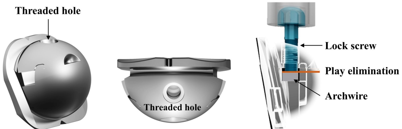
Fig. 1 Design of the spherical self-ligating bracket with the lock-hook system
