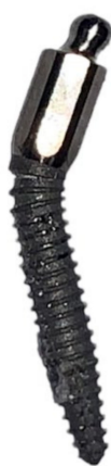
Figure 4. Retrieved mini dental implant sample from the resin block following testing, showing the bend under the first thread.
