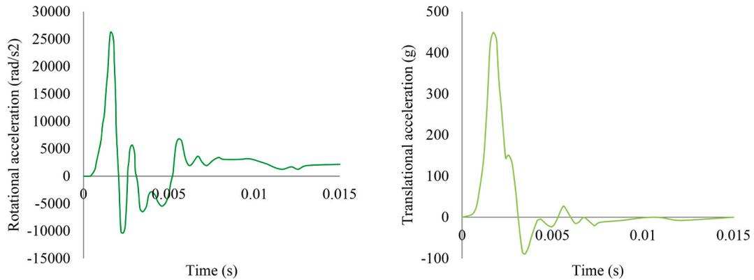
**Fig. 4.** Head loading conditions employed in the impact study: Left Panel: rotational acceleration and Right Panel: translational acceleration.
