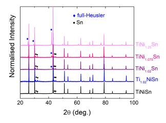
**Figure 1.** Laboratory X-ray (Cu  $K_{\alpha 1}$ ) powder diffraction patterns for the TiNi<sub>1+y</sub>Sn series and Ti<sub>1.02</sub>NiSn. Data are normalised and offset along the intensity axis and plotted against 20 angle.
