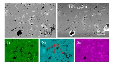
**Figure 4.** Backscattered electron (BSE, left) and secondary electron (SE, right) SEM images and EDX maps (Ti, Ni, and Sn respectively) for  $TiNi_{1.02}Sn$ . The elemental maps cover the same area as the BSE and SE images.
