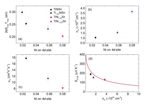
**Figure 6.** (a) Thermal band gap  $(E_g)$ , (b) Hall carrier concentration  $(n_H)$ , and (c) Hall mobility  $(\mu_H)$  versus Ni-4d site occupancy. (d) Pisarenko plot using a single Kane band with carrier effective mass  $m = 2.8 \text{ m}_e$ .
