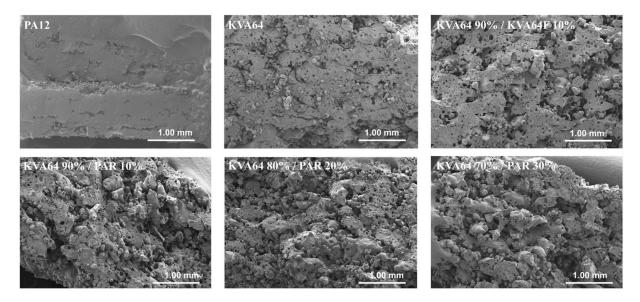
**Figure 8.** SEM images of the SODFs vertical sections (Magnification ×30).
