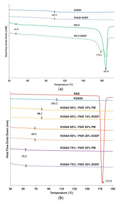
**Figure 4.** DSC curves: (**a**) KVA64 and PA12 before and after sintering (**b**) KVA64, paracetamol, physical mixtures and sintered SODFs.
