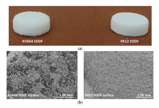
**Figure 7.** General aspect of KVA64 and PA12 SODFs printed at optimal parameters: (**a**) Images of the SODFs, (**b**) SEM images of the SODF surfaces (Magnification ×30).
