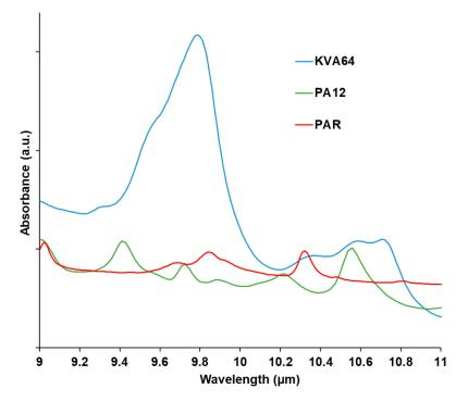
Figure 3. FTIR spectra of KVA64, PA12, and PAR from 9 to 11  $\mu$ m.
