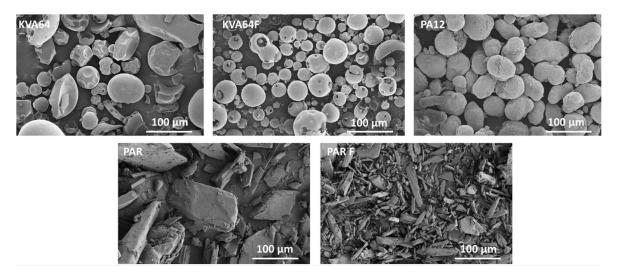
Figure 2. SEM images for KVA64, KVA64F, PA12, PAR, and PAR F powders.
