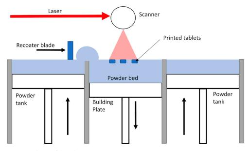
Figure 1. Schema of the Selective Laser Sintering process.
