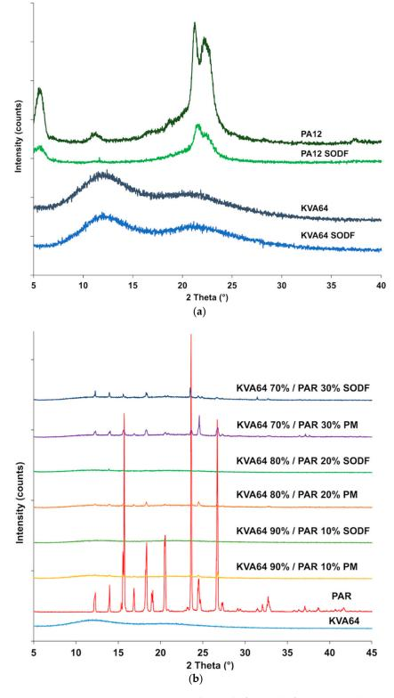
**Figure 6.** XRPD patterns: (**a**) KVA64 and PA12 before and after sintering (**b**) KVA64, paracetamol, physical mixtures and sintered solid oral dosage forms (SODFs).
