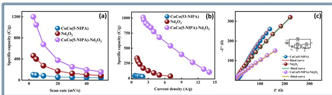
Fig. 5 (a) Specific capacities of CuCo(5-NIPA), Nd<sub>2</sub>O<sub>3</sub>, and CuCo(5-NIPA)-Nd<sub>2</sub>O<sub>3</sub> through CV analysis. (b) Specific capacities of CuCo(5-NIPA), Nd<sub>2</sub>O<sub>3</sub>, and CuCo(5-NIPA)-Nd<sub>2</sub>O<sub>3</sub> through GCD analysis. (c) Comparison of the electrochemical impedance spectroscopic curves for CuCo(5-NIPA), Nd<sub>2</sub>O<sub>3</sub>, and CuCo(5-NIPA)-Nd<sub>2</sub>O<sub>3</sub> along with the fitted curves.
