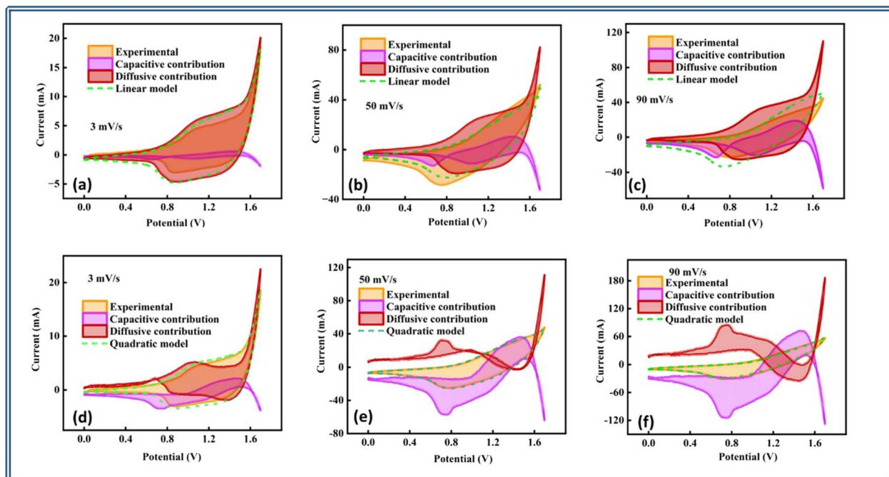
Fig. 8 Capacitive diffusive contributions at 3, 50, and 90 mV s<sup>-1</sup> obtained through the (a)–(c) linear model and (d)–(f) quadratic model.
