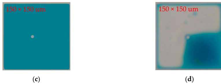
Figure 1. Principle of the electrowetting display (EWD). (a) Without applied voltage, the color of oil is displayed in a pixel. (b) With applied voltage, the color of substrate is displayed. (c) The top view when the pixel is turned off. (d) The top view when the pixel is turned on.
