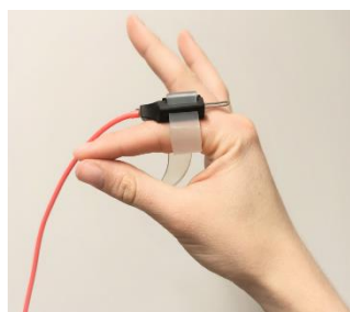
Figure 1. Accelerometer positioned at the base of the right index finger.
