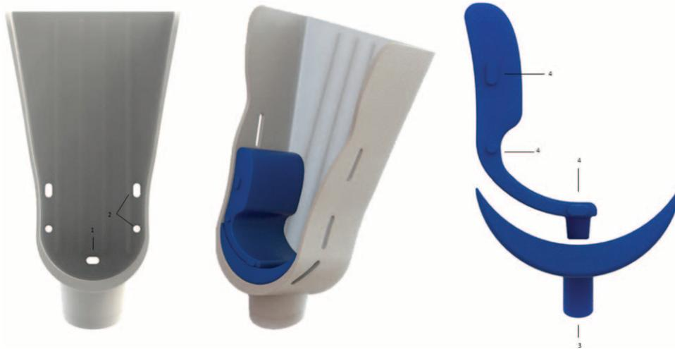
**Figure 5.** Adjustable foot base to enforce an internal or external rotation. The foot base has 2 components that fit in notches at the foot platform. (1) Inferior and (2) side pin fitting for the adjustable foot base; (3) inferior silicon pin that fits into the foot platform; (4) inferior silicon pin that fits on top of the inferior component of the adjustable foot base and lateral silicon pins that fit in the lateral borders of foot platform.
