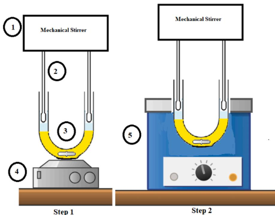
**Fig. 2.** Schematic of recycling setup for ILM with deionized water; (1) mechanical stirrer with controlled speed, (2) glass stirrer rod, (3) magnetic bar, (4) magnetic stirrer, and (5) ultrasonic bath.
