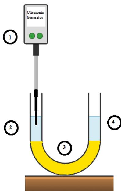
**Fig 1.** (1) Ultrasonic probe, (2) feed phase, (3) membrane phase, and (4) receiving phase.
