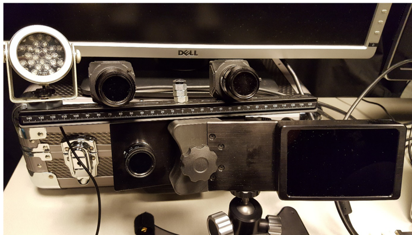
Fig. 5 Experimental setup for the validation study. The stereo tracker was mounted on top of the EyeLink camera
