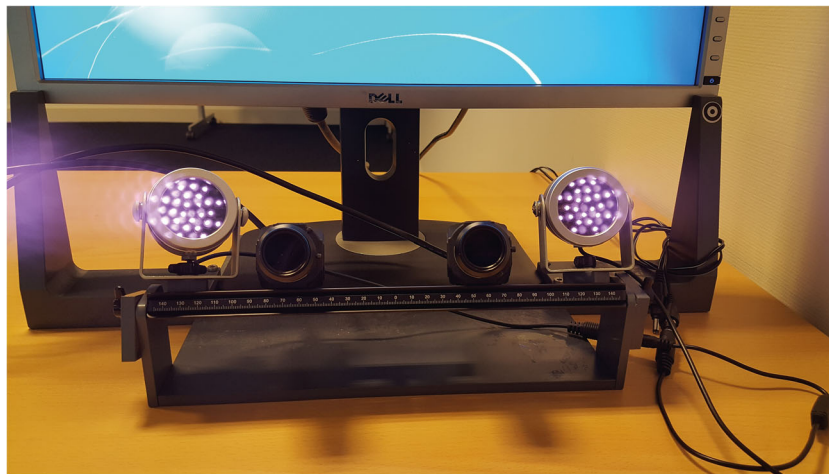
Fig. 1 The stereo eyetracking system. The hardware consists of two infrared illuminators and two USB 3.0 cameras connected to a laptop computer
