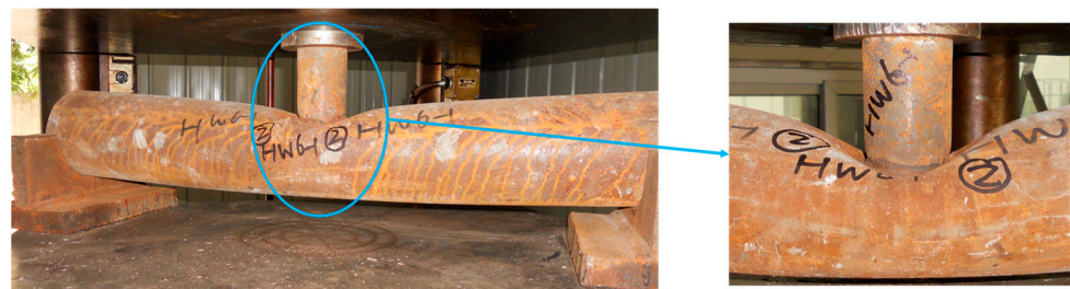
Figure 7. Typical failure mode of hollow steel tubes under bending [19].
