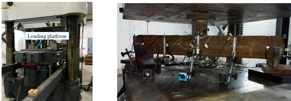
Figure 4. Layout of loading platform.
