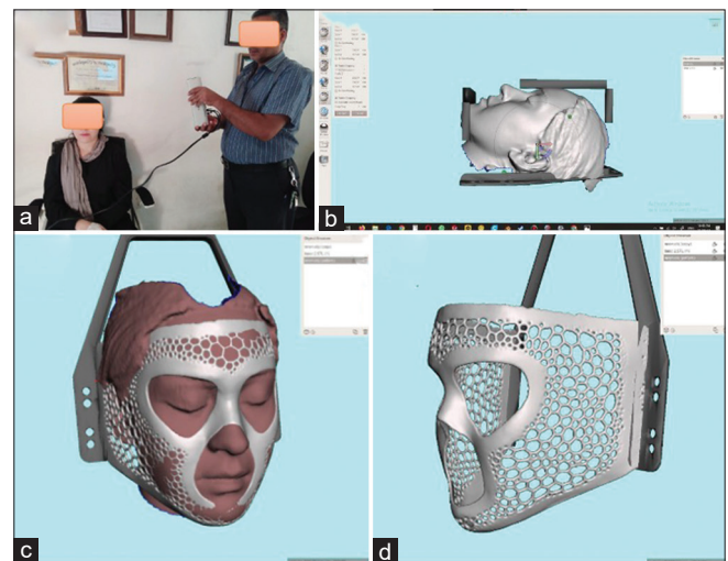
Figure 3: (a) A digital scanner takes a 3D-shaped patient's head. (b-d) The data were manipulated with Meshmixer software to design patient-specific masks. The mask produced is porous to reduce the material and the time to form it.
