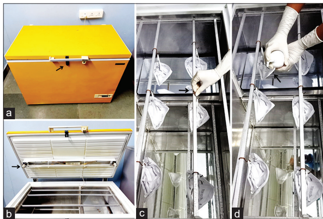
Figure 1: (a) Image of the old condemned airtight freezer box. An additional lock (black arrow) is provided as a safety feature. (b) Image of the freezer box with open lid depicting installed UV-C light (254 nm- black arrow) for decontamination of respirators. (c) Image of the open freezer box depicting how respirators are attached with the help of copper hangers (black arrow). Additionally the mirrors can be seen on the base and the walls of the box for reflecting UV-C light. (d) Image depicting how hydrogen peroxide is sprayed over the respirators (black arrow) before switching on the freezer box
