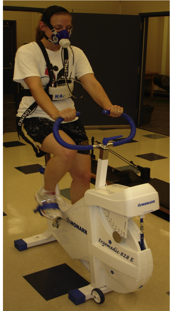
Figure 2. The Monark Ergonomic 828 E Bicycle Ergometer.
