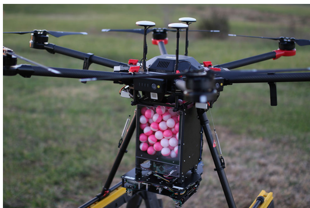
Fig. 7 A hexacopter equipped with a system to disperse self-igniting balls for starting controlled fires, as reported by [59]. Photo by courtesy of Drone Amplified Inc
