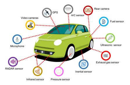
Figure 1. Different types of in-vehicle sensors.
