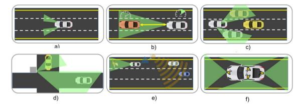
**Figure 5.** An example of ITS safety applications: (**a**) lane keeping aid, (**b**) adaptive cruise control, (**c**) blind spot information, (**d**) intersection collision warning, (**e**) road hazard warning and (**f**) surround view monitoring.
