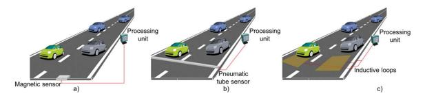
**Figure 2.** Intrusive sensor groups, (**a**) Embedded magnetometers, (**b**) Pneumatic tube sensors and (**c**) Inductive loops.
