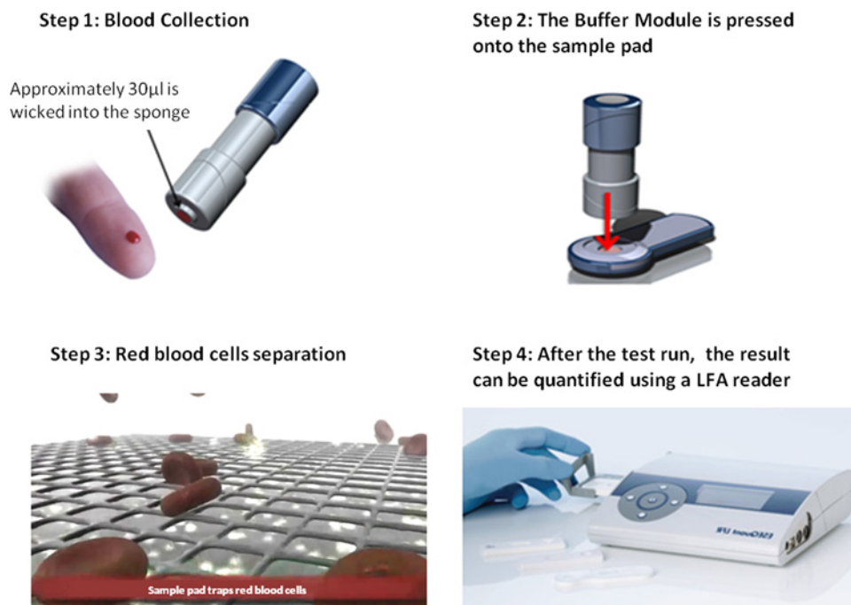
Figure 4. An example of an integrated sample collection device combined with a cassette and strip reader
