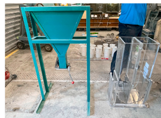
(c) V funnel and U box apparatus
