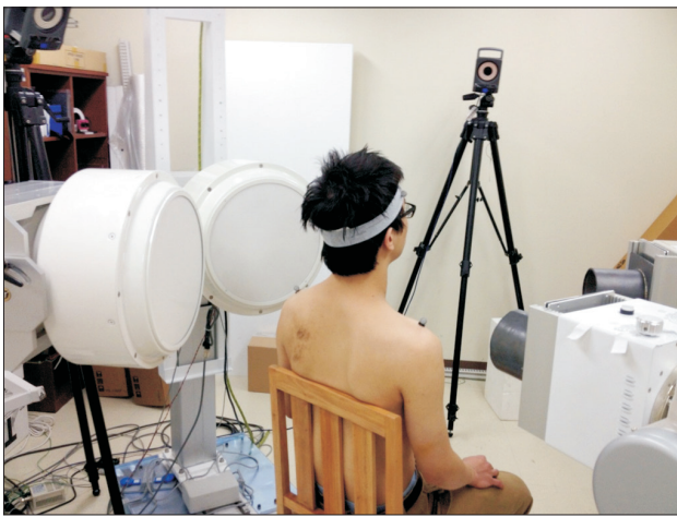
Fig. 1. Biplanar fluoroscopic images aligned horizontally and angled at approximately 55° were collected from a system composed of two focal-spot radiograph tubes (KMC-1400ST; COMED Technologies Inc., Gwangju, Korea).
