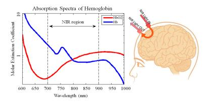
Figure 1. A schematic of how the fNIRS works with the absorption spectra of *HbO2* and *Hb*.
