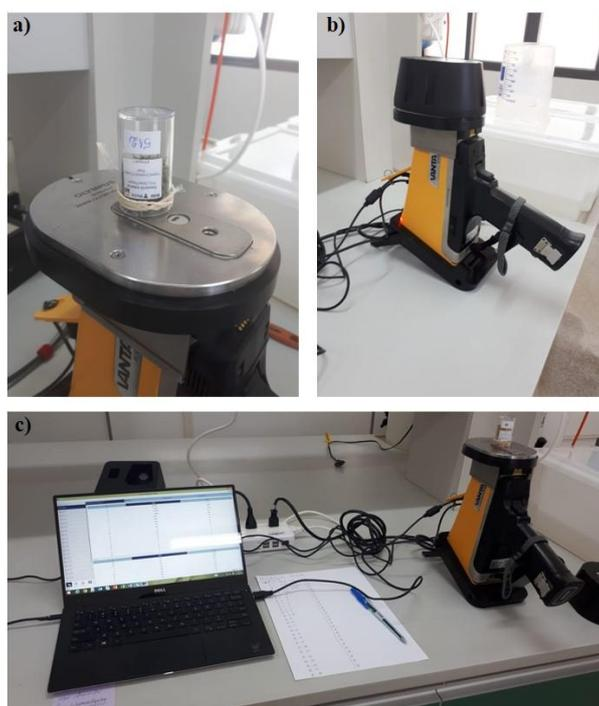
**Figure 2.** Details of portable X-ray fluorescence (pXRF) measurements. (a) Detail of ground leaf sample into the plastic vial and placed on X-ray source and detector aperture; (b) samples covered by a proper cap for protection against the X-ray; (c) data acquisition in real-time using a laptop connected to pXRF equipment.
